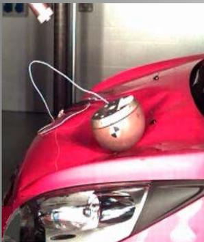
Vehicles are now tested for pedestrian style impacts on the front end of the vehicle. This involves a series of tests on different zones on the vehicle and at level levels of impact. You can see videos of these tests at MIRA [Here](#)
